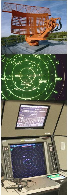
*Top:* An ASR-9 radar antenna. *Middle:* ATC radar screen, 1950s, similar to the display used by the author in testing.
